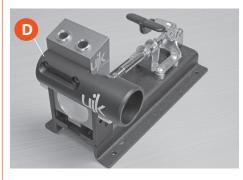
Locate the dust extractor assembly and the two Hex screws (**D**). Line up the pre-drilled holes with the threaded holes to the front of the guide block and secure with the two Hex screws.
