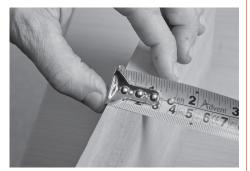
**Step 1** Measure the width of the timber, see picture above.
