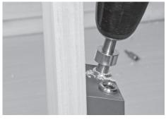
**Step 6** Remove the drilled pocket hole joint from the jig, see diagram below.
