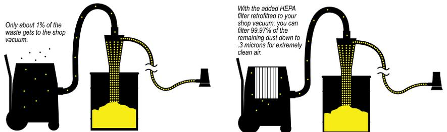
**Cyclone separates 99% of the dust before it reaches your shop vacuum. No filter clogging and no loss of suction.**
