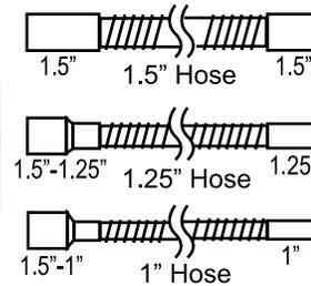
All hose is high quality, static dissipating, wire reinforced.
