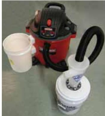
2nd Pail Bolted to Barrel of Wet/Dry Vacuum.
