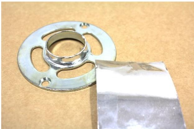
If your copy ring is too loose, add a strip of aluminium tape (included in the package) around your ring, covering the whole ring. Do not use too much tape as it might start warping upwards, this will give a tight, but offset fit.
