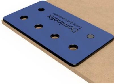
Flip the jig around and put in place with the bench dogs (included in the package) in the row you routed first. Make sure you don't have any play on the jig, this will cause imperfection while you are copying the pattern.
