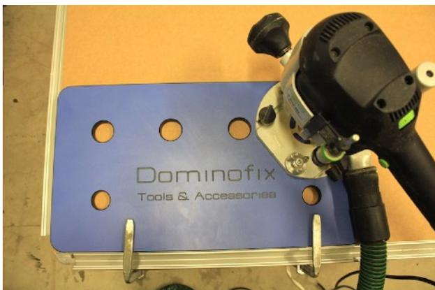
Place the jig on your worktop to route the first set of holes. The outside measurements of the jig allows you to recreate the same starting distance from the edge till the first holes as a Festool MFT top.
